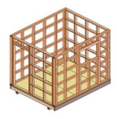
Lift and Fix the Wall Frames in Place
