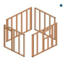
Make the Wall Frames up on even ground, referring to the <u>'Wall Frame and Stud Placement'</u> Plan which shows the placement of the studs from a bird's eyeview. In this particular plan, the Studs are spaced at 600 [2ft] crs or o.c.(which means "at centers" or "on center"). This means the Studs are spaced apart 600 (2ft) from the center of one Stud, to the center of the adjoining Stud (where possible).
